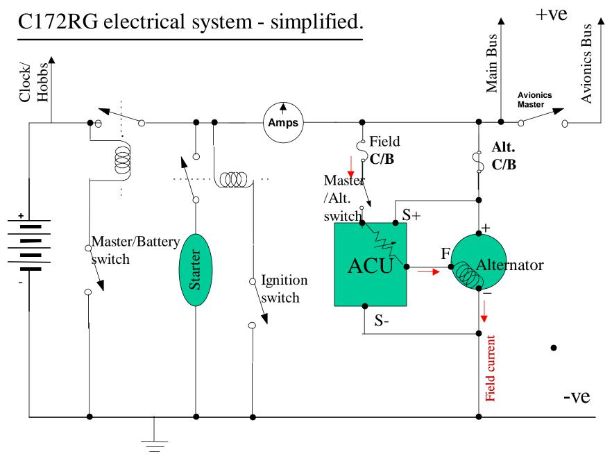
The ACU adjusts the field current to maintain the alternator output S+ - S- at 28.4V.
