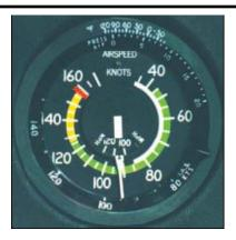
Lift (and drag) are proportional to air\_density \* TAS<sup>2</sup> i.e  $\rho v^2$ As the air density drops with altitude, we must increase our TAS (by 1.6%/1000 ft) to maintain the same lift, all else equal (i.e. identical configuration, AOA etc.).
