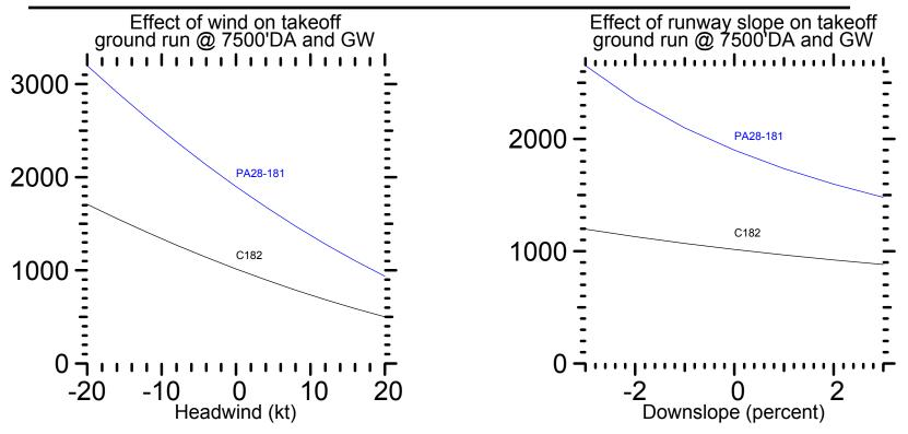
Ground roll decreases about 6% per thousand feet of ground roll for each percent of downslope. (Same **increase** for landing ground roll.) Ground roll varies as the square of your liftoff ground speed.
