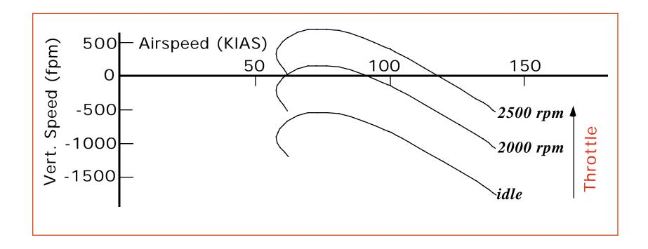
★ Reduction of power by  $_{500RPM/5''}$  MP => 500 ft/min descent
