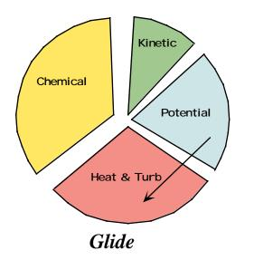
In a constant airspeed, power-off glide, potential energy (altitude) is dissipated by drag. Kinetic and chemical energy are constant.
