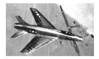
Pilots enhanced low-speed controllability of F-100 by lodging elbows in side of cockpit to neutralize ailerons
