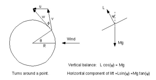
Centrifugal Force= Component of horizontal component of lift towards center  $Mw^2/R = Mgtan(\psi) \cos(\phi)$
