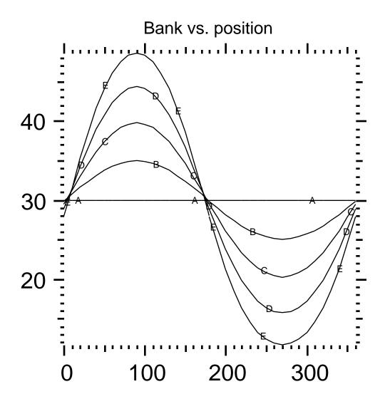
Here we look at a turn which requires a 30 degree bank in no wind. Curves A,B,C,D and E are with no wind and with winds of 10%, 20%, 30% and 40% of the TAS respectively. At the 90 and 270 points the plane is directly downwind and upwind respectively. At 0 and 180, the plane is
