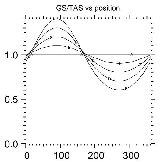
We now show bank angle vs. gs/TAS for a turn that requires a 30 degree band in no wind. Curves A, B, C and D are for winds of 10%, 30%, 50% and 70% of the TAS. We see that the required bank angle is primarily determined by the ground speed. However, there is the effect, decribed earlier, that as the wing gets stronger the crab angle increases, so that a smaller fraction of the horizontal component of lift is directed towards the center of the turn.
