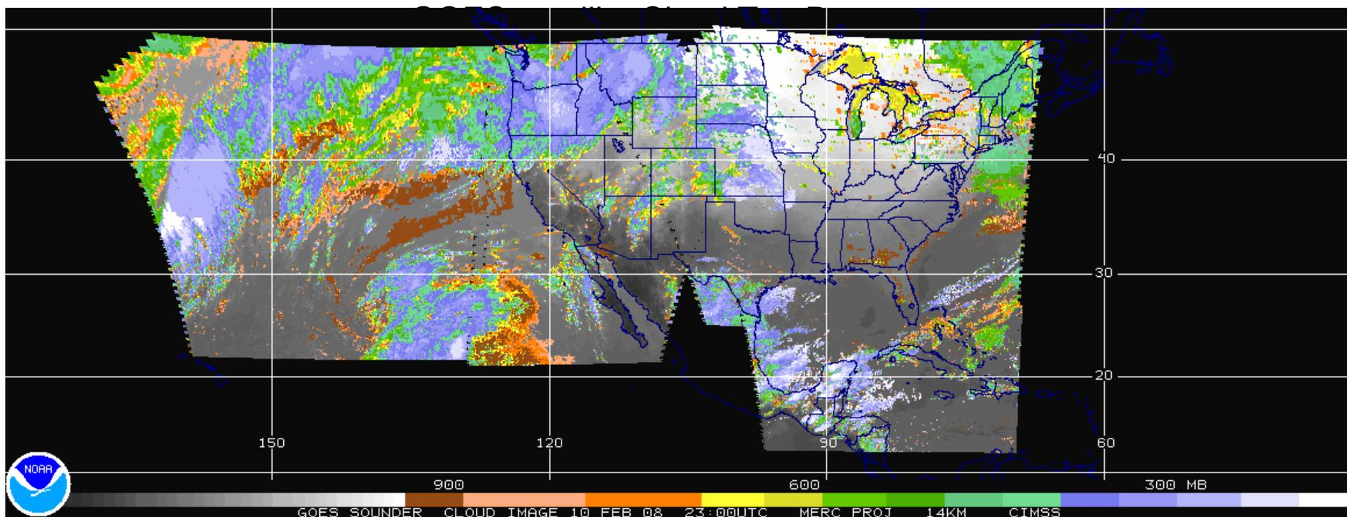
This product derives cloud top heights from IR spectral measurements from the GOES satellites.
