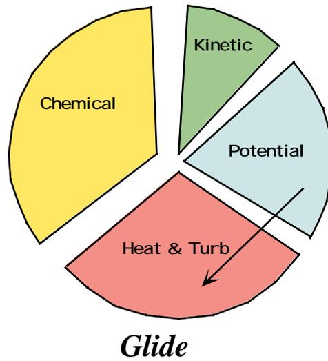
In a constant airspeed, power-off glide, potential energy (altitude) is dissipated by drag. Kinetic and chemical energy are constant.
